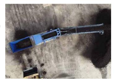
Fitted with a remote operated 180° radial discharge conveyor as standard, the EDGE FTS Radial stacker has a maximum discharge height of 6m (19'10") facilitating the creation of stockpile capacities of up to 952m³ (1246yds). Added versatility is provided by the FTS Radial's ability of continuous stockpiling whilst tracking, giving operators the ability to increase their stockpile holding capacity over a much smaller footprint.
