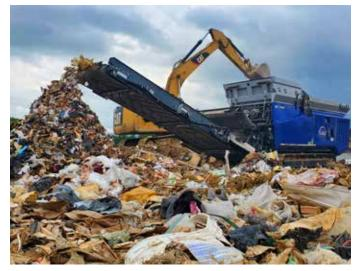
The shredder chamber is controlled via the latest EDGE Operating System (EOS) which is designed for improved user-friendly controls and gives operators greater control over program settings, shaft speed and reverse cycles. The VS420 operating system provides 5 factory set shredder programs for demolition wood, general waste, green waste, mattresses, and compost. There are 3 additional program settings that can be tailored by the operator to suit their specific input materials.
